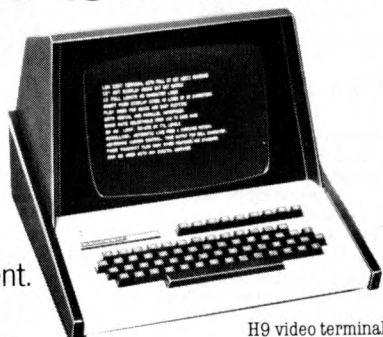
H9 video terminal, with 67 ASCII keys.
